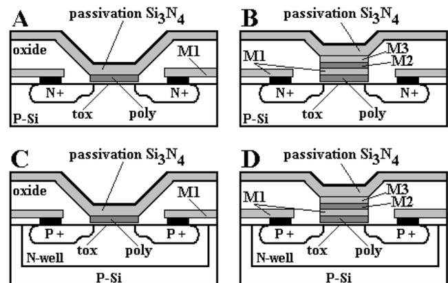
Fig. 3. Cross sections of the ISFET gate structures implemented in the submicron CMOS technology (M1=metal1, M2=metal2, M3=metal3 layers); not in scale.
