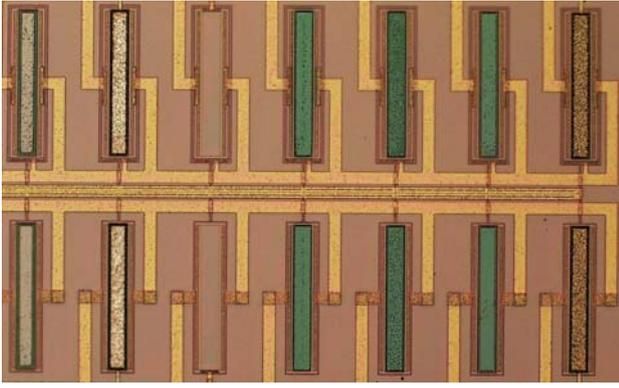
Fig. 5. Detail photo of some N and P-type ISFET microsensors, the gate area of each device is 250/30 $\mu$ m.
