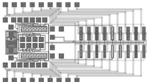
Fig. 4. Layout of the CMOS ISFET experimental structures.
