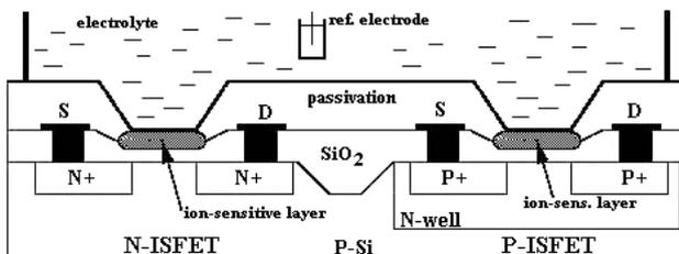
Fig. 1. Schematic cross section of N and P-type ISFETs in CMOS technology.
