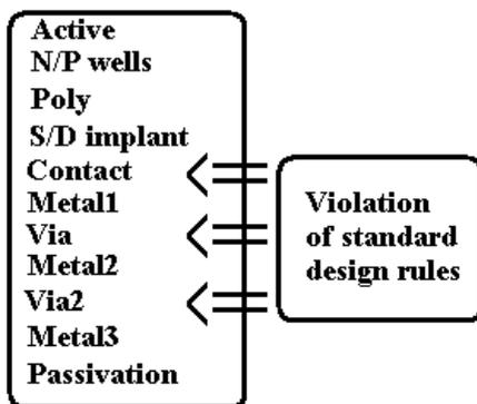
Fig. 2. Graphical representation of the CMOS process mask flow with required design rule violations for ISFET sensor designs.
