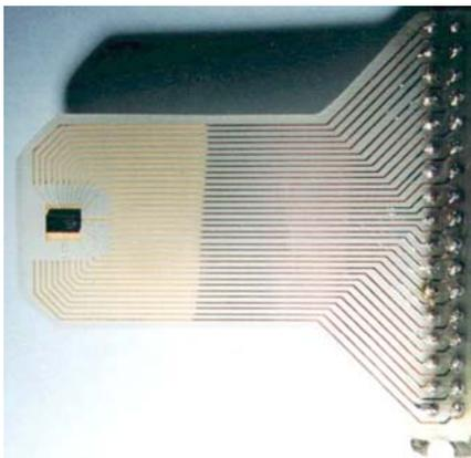
Fig. 6. PCB test probe for ISFET sensor chips before encapsulation.
