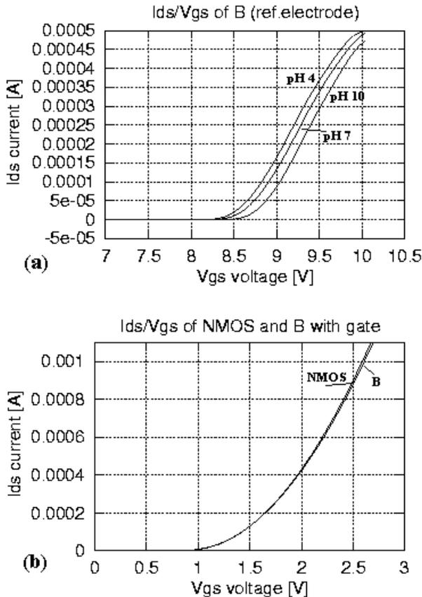
Fig. 8.  $I_{gs}/V_{gs}$  characteristics of B sample with the Ag/Cl reference electrode with floating Al gate (a), and  $I_{ds}/V_{gs}$  comparison between the same sized NMOS and B sensor when a same  $V_{gs}$  is applied on its Al gate (b),  $V_{ds}=5V$  in both curves, at room temperature.
