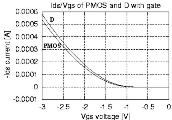
Fig. 9.  $I_{ds}/V_{gs}$  comparison of D structure and the same sized PMOS with  $V_{gs}$  applied on their gates,  $V_{ds}=-5V$ , at room temperature.
