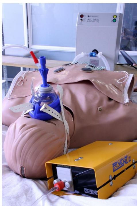
Figure 1 Experimental setup when ASL 5000 did not performed well. High frequency jet ventilation of a patient
