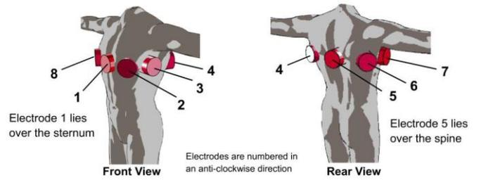
Fig. 1. Electrode positions for measuring using EIT system Maltron Sheffield Mk 3.5 [Maltron Sheffield Mk 3.5 user manual, 2008].
