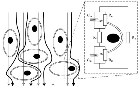
Fig. 2. Current passage through tissue and electrical analogy of the cell [9].
