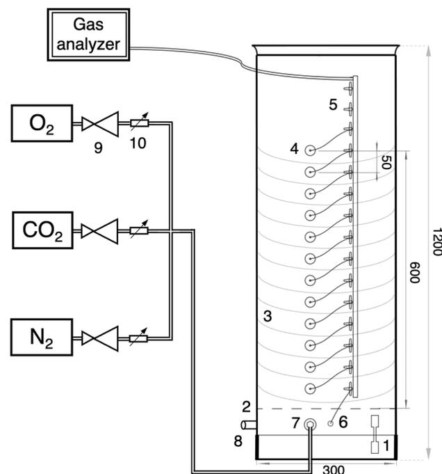
**Figure 1.** A scheme of the apparatus with the gas analyzer and gas cylinders. 1—buckle fixing the cover to the cylinder; 2—plastic mesh separating the cylinder into two parts; 3—airtight O-rings; 4—rubber plug with a metal needle; 5—three-way valve; 6—sampling point of the gas mixture in the inlet chamber; 7—gas inlet port; 8—gas outlet port; 9—pressure-reducing valve; 10—throttle valve. Dimensions are in millimeters.
