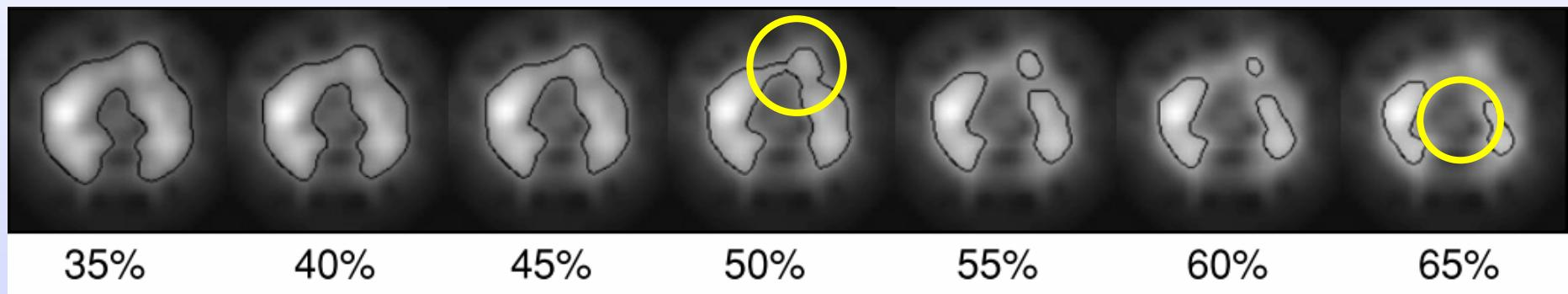
Standard deviation of relative impedance change of each pixel.
