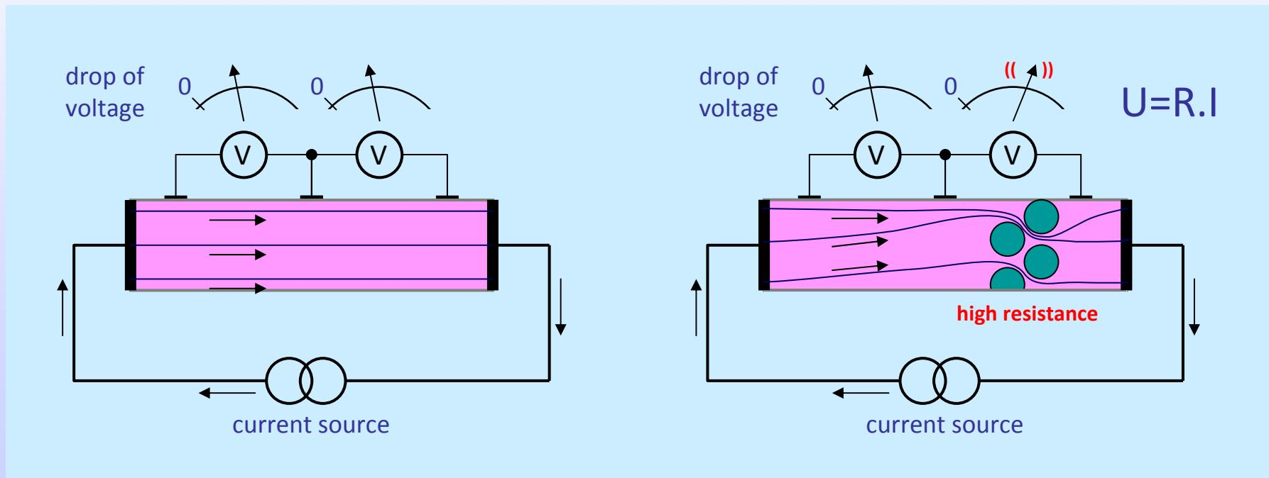
**Principle:** Measurement of impedances (resistances) of the lungs at different angles with a consequent image reconstruction similar to CT.
