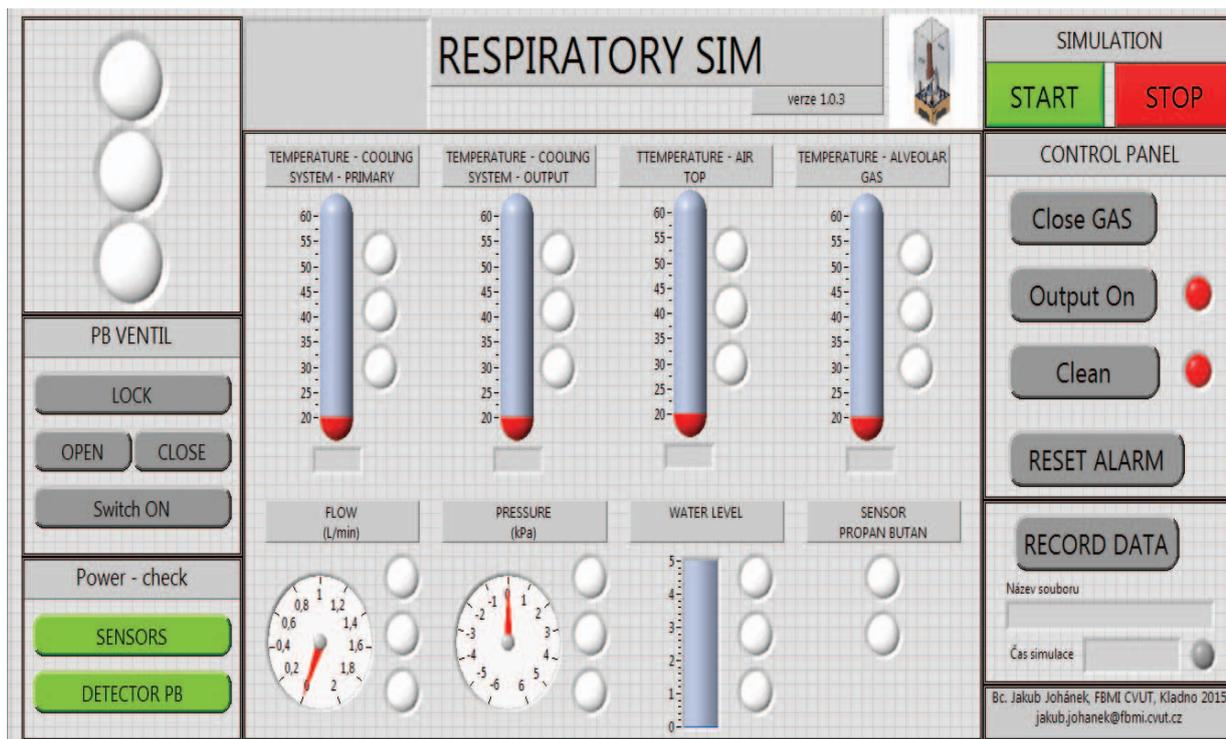
Fig. 2. Control panel. On the panel there are displayed information from all sensors in the interior of the simulator.
