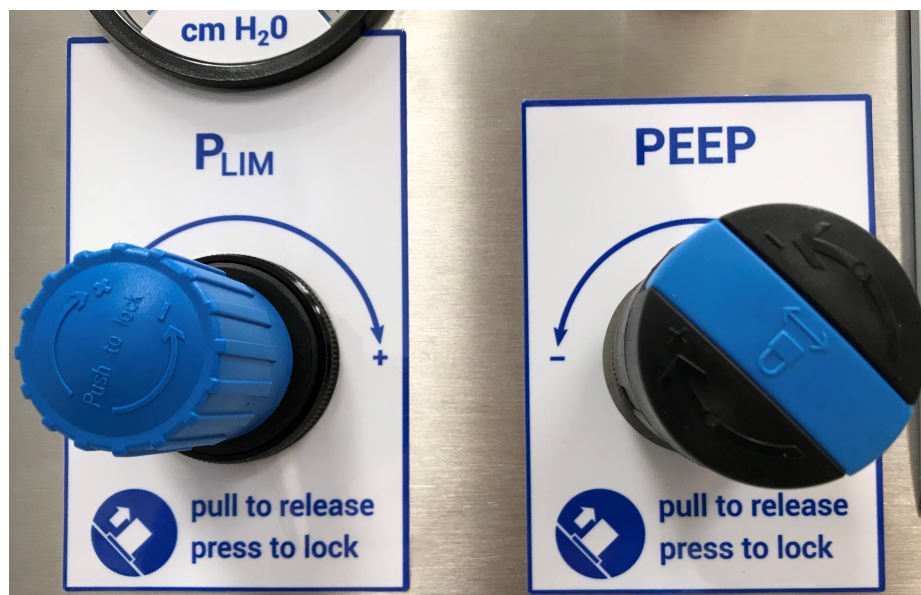
Fig. 11: Rotating controllers for ventilation parameter setting – Plim (left) and PEEP.
